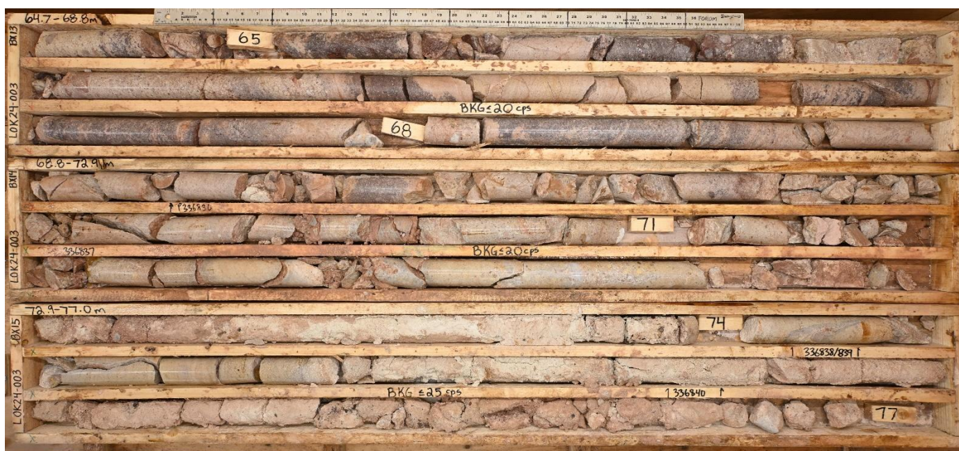
Figure 4 Core photo of LOK24-003 showing the intense clay alteration in the sandstone around 70 m.
